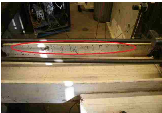
Figure 4.39: N col. initial yielding at +1.4\% drift (Y1-OF).
