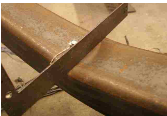
Figure 4.78: S brace cupping at 3.0% drift (B3-PH).
