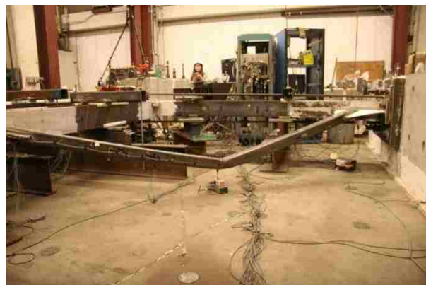
Figure 4.53: N brace buckling at 3.3% drift (B3-PH).
