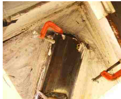
Figure 4.36: Mid-span GP yielding at -0.83% drift.
