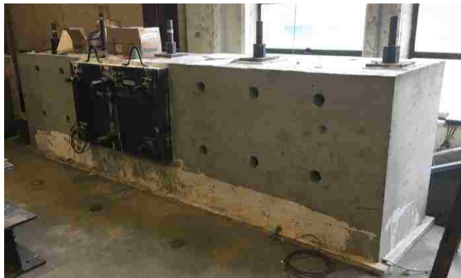
Figure 3.2: Reaction block used for N column anchorage.
