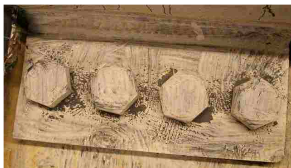
Figure 4.86: Shear tab moderate yielding at +3.3% drift (Y2).
