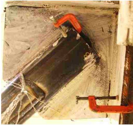
Figure 4.41: GP yielding at 1.7% drift (Y1).
