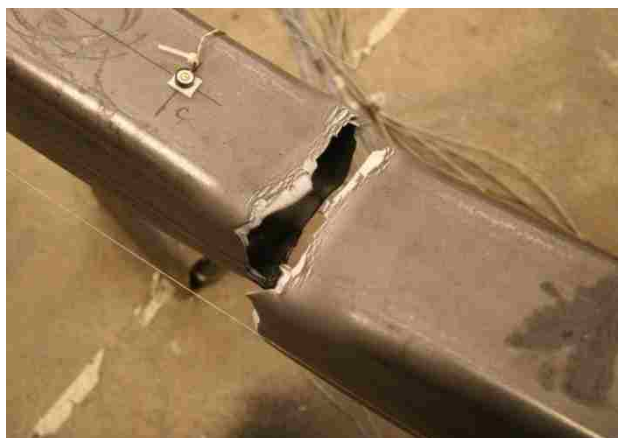
Figure 4.24: S brace fracture at second cycle of +3.0% drift (B4-BF).
