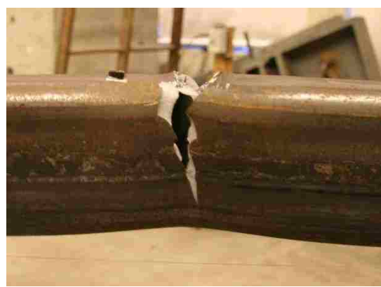
Figure 4.85: S brace \frac{3}{4} tear at 3.6% drift (B3-BT).
