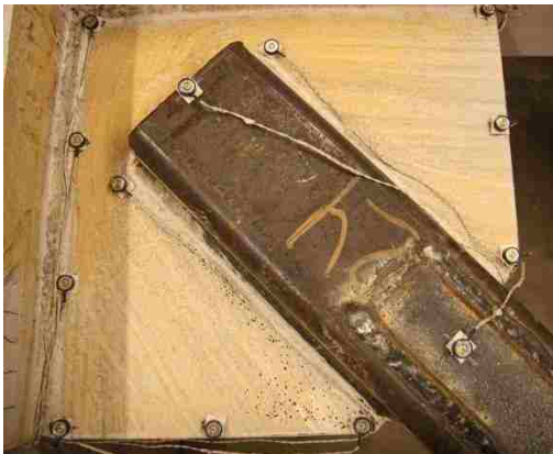
Figure 4.63: Mid-span GP initial yielding at 0.4% drift (Y1).
