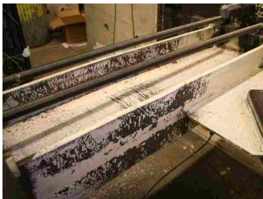
Figure 4.76: N col. severe yielding at 2.8% drift (Y3-PH).
