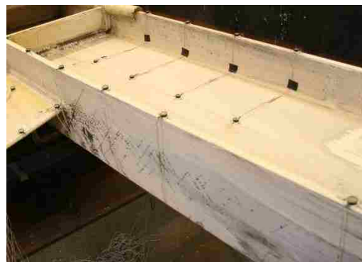
Figure 4.73: Beam IF yielding at 1.9% drift (Y1-OF).
