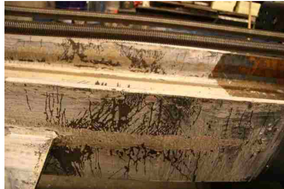
Figure 4.14: S col. moderate yielding at -1.9% drift (Y2-PH).
