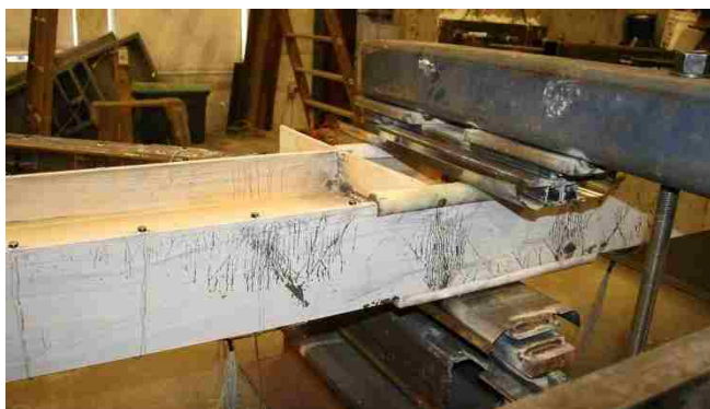
Figure 4.72: Beam OF yielding at 1.9% drift (Y1-OF).
