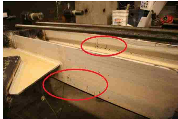
Figure 4.69: S col. initial yielding at 1.4% drift (Y1-OF/IF).
