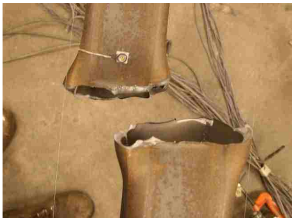
Figure 4.88: N brace fracture at -3.6% drift (B4-BF).
