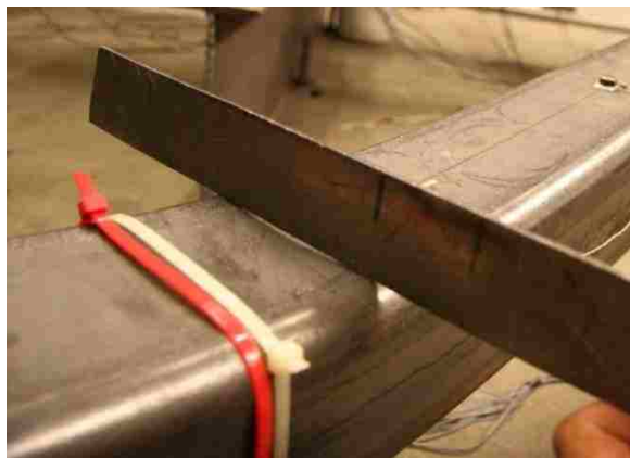
Figure 4.15: S brace initial cupping at -1.9% drift (B3-PH).
