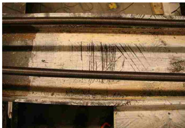
Figure 4.17: Initial local buckling in N (left) and S (right) column flanges at +2.2\% drift (LB1-OF/IF).
