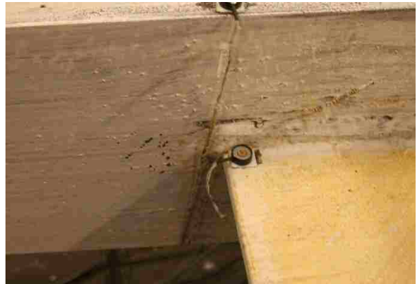
Figure 4.64: Initial yielding in beam IF at 0.41% drift (Y1-IF).
