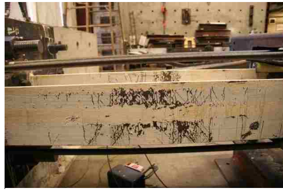
Figure 4.44: N col. moderate yielding at 1.9% drift (Y1-OF/IF).
