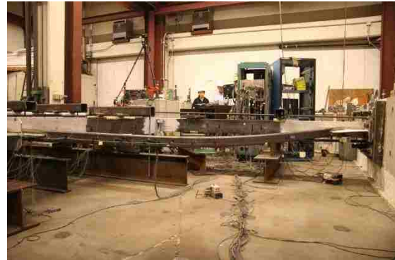
Figure 4.34: N brace buckling at 0.41% drift (Y1).
