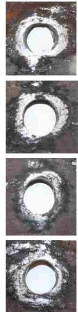
Figure 4.57: N beam web bolt hole elongation.
