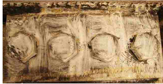
Figure 4.66: S shear tab yielding at -0.83% drift (Y1).
