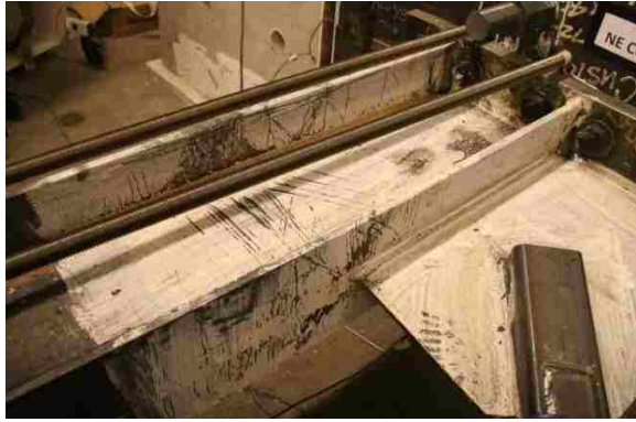
Figure 4.13: N col. moderate yielding at +1.9% drift (Y2-PH).
