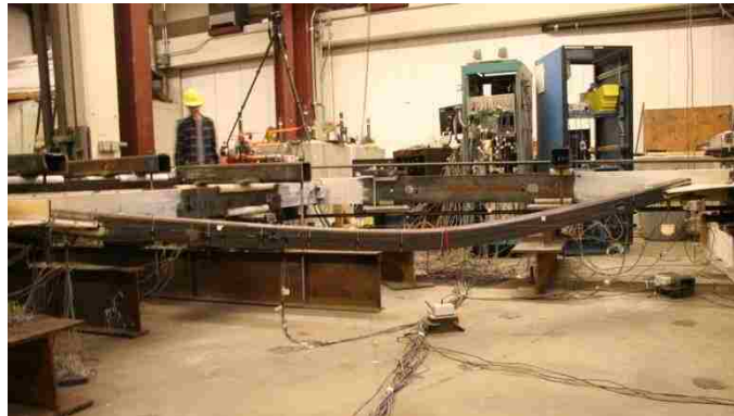
Figure 4.67: N brace buckling at +0.83% drift (B2).
