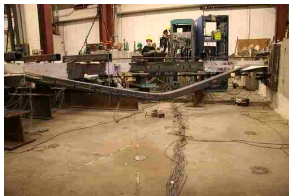
Figure 4.46: Brace buckling at 2.5% drift (B1).
