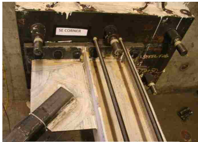
Figure 3.8: Base plate attached to interface plate.
