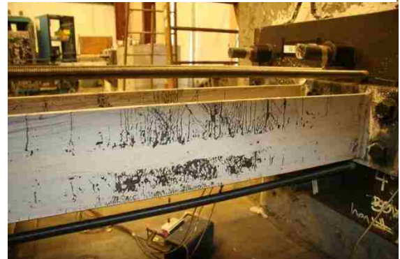
Figure 4.71: S col. moderate yielding at 1.9% drift (Y2-PH).
