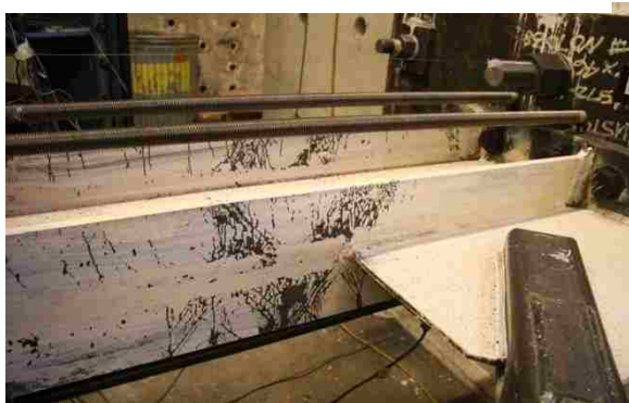
Figure 4.70: N col. moderate yielding at 1.9% drift (Y2-PH).
