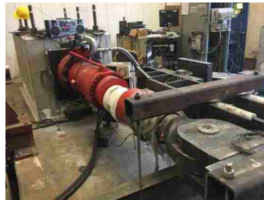
Figure 3.3: Hydraulic actuator and reaction block.
