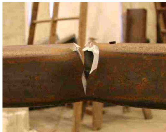
Figure 4.83: N brace \frac{3}{4} tear at -3.3% drift (B3-BT).
