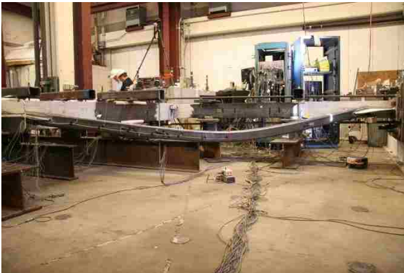
Figure 4.37: N brace buckling at +1.1\% drift (B1).
