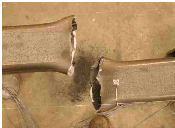
Figure 4.89: S brace fracture at +3.6% drift (B4-BF).
