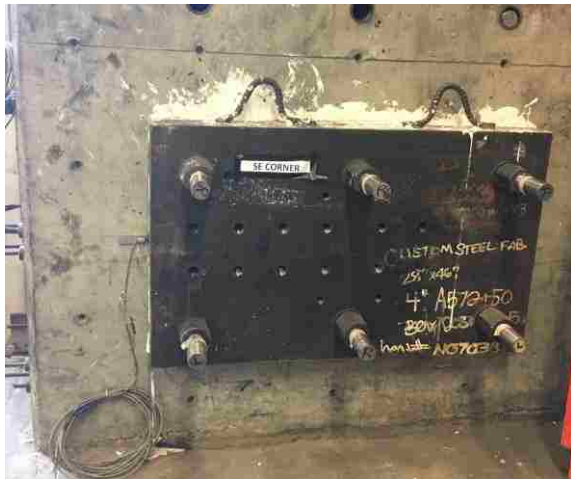
Figure 3.7: Interface plate attached to strong wall.
