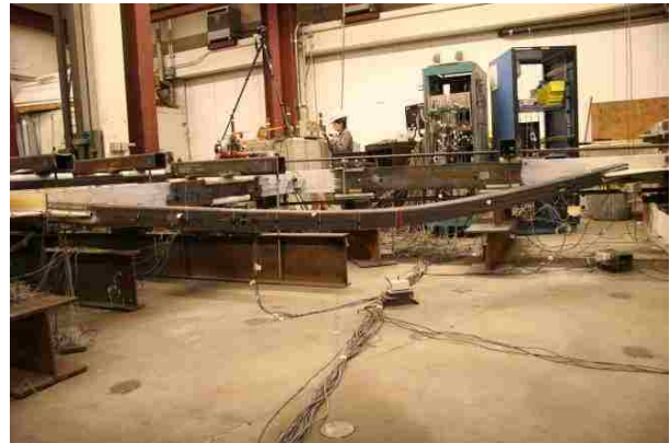
Figure 4.62: N brace buckling at 0.7% drift (B1).
