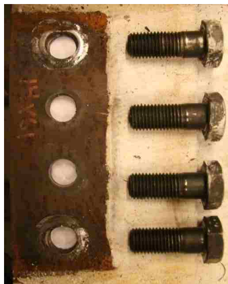
Figure 4.56: S beam web bolt hole elongation.
