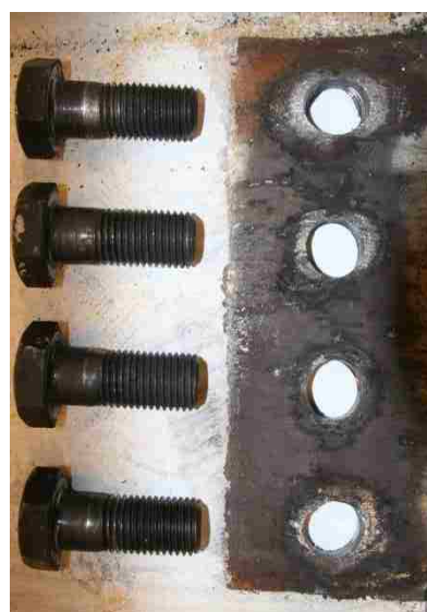
Figure 4.57: N beam web bolt hole elongation.
